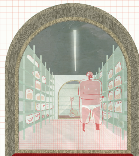
View from the incubator. This is the last step of the growing process. The mycelium grows and eats the plant substrate. This room needs to be dark and sterile. After passing the mycelium in the mold, the proliferation process takes three weeks. After this period, the point is ready and can go upstairs, to be palletized and transported to building site.
