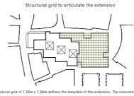
A structural grid of 7,00m x 7,00m defines the template of the extension. The concrete structure (which can be prefabricated) with high load capacity slabs makes possible to accommodate a secondary structure that will divide and organise the double-height of the main structure. This
