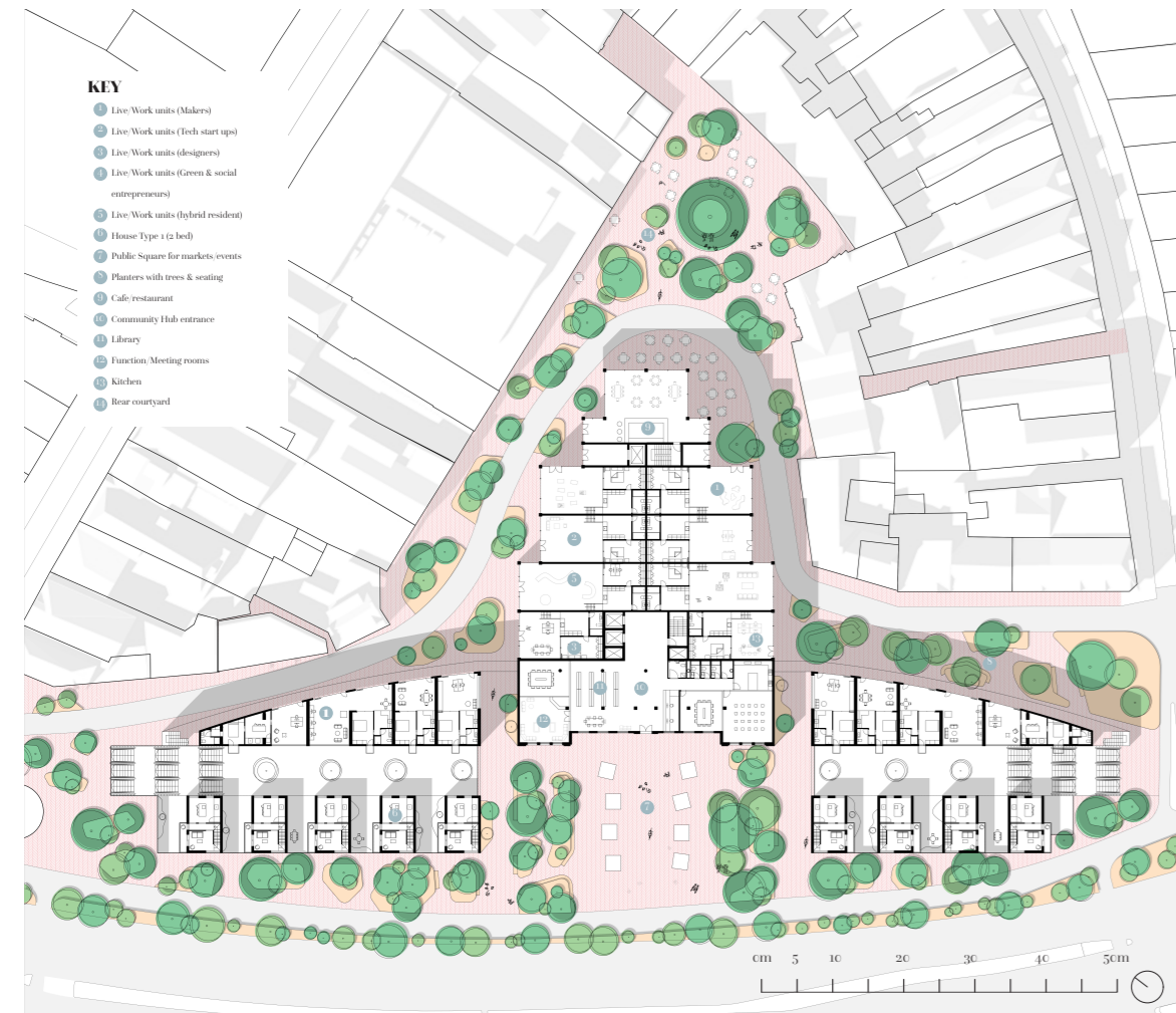
A row of small detached houses is introduced to perforate the southern façade, bringing human scale and street-level activity, while also increasing floor area. The two existing wings are topped with a lightweight timber-framed storey, featuring chamfered roofs that respond to the surrounding context. In the courtyard, perforated modules are supported by new perimeter columns to create an open, welcoming façade. Cantilevers and balconies animate the edge, offering moments for informal interaction and social exchange.
