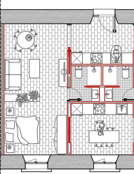
SIMPLEX units (37.5m 2 each) South Block / e 1:100 The studio-homes always guarantee cross ventilation and natural light, with the kitchens serving as the connecting point for potential future expansion.
