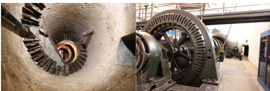
A gallery allowed the water from the old turbine to flow out into the Broquetas drainage channel. A set of manual gates installed in 1950 allowed the water from the Planas turbine to be diverted to a new Francis turbine, which used the small difference in height between the gallery and the outer channel to harness the power of the water.
